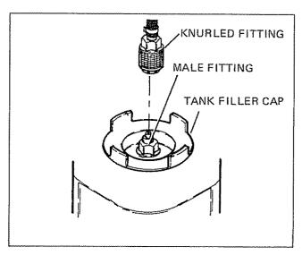
2. To connect fuel line quick-disconnect to tank fitting, pull back on quick-disconnect knurled fitting. Insert open end of knurled fuel line fitting over male fitting on tank, then let knurled fitting snap into place to lock.
